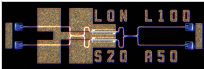
Phase shifters for the optical gates
