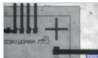
Fig. 3 Infrared image of a joined hybrid foil system with nano contacts.
