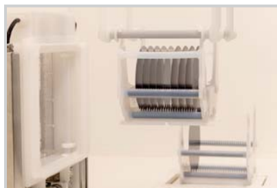
Simultaneous automatic processing of 150 mm and 200 mm substrates
